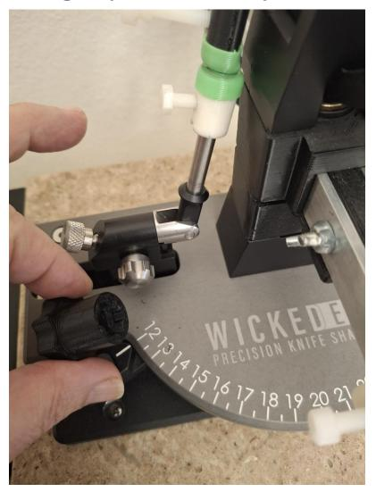
These larger snap-on knobs allow you to tighten the screw in the rear of the adjuster so there is more tension on it to allow you to move the adjuster with ease but in a more controlled manner. This allows faster angle setting with less repeated back and forth movements to get angle exact. Just pop off the WE provided plastic covers and push on the Big Wheels!
