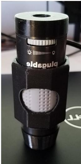
Microscope User's Kit: provides protected ready access to focus ring and shutter discharge. Avoid constant refocusing at high power. Lens shroud cover provides glare shade, knife edge cut protection, improved bevel position and hold, w/indexing notch. \$16/Kit
