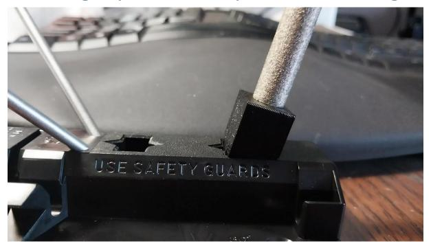
The adapter uses the Spyderco Original Sharpmaker's selected angle with Jende diamond round rods to allow a serrated knife to be hand-held sharpened with this popular guided system.
