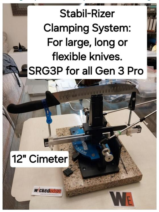
Stabil-Rizer Clamping System for Gen 3 Pros: SRG3P \$120
