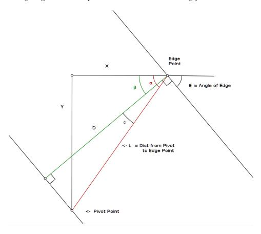
In this diagram L is the distance from the edge point (where we are evaluating) to the pivot point, again, considering ONLY the in-plane horizontal and vertical directions. These are in the figure as the line lengths X and Y respectively. (Remember that the real pivot point is a distance O outside the mounting plane). To begin
